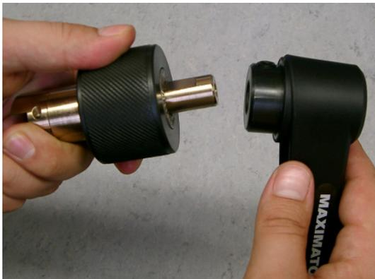
Stick the components onto the blanking die holder in the following sequence: Needle bearing → Knurled nut → Needle bearing → Crank handle.
