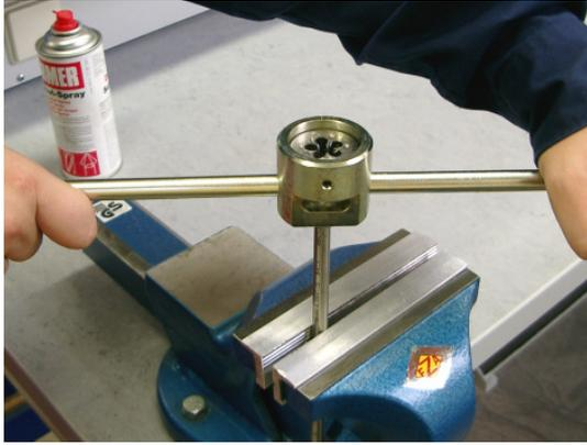
Slightly press down the tool and start the threading operation (in counter-clockwise direction). Rotate the tool briefly in clockwise direction during the threading process in order to break the chip and apply more cutting oil.
