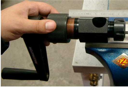
Turn out the knurled screw until only ca. 2 – 3 thread turns are gripping. This corresponds to a distance of 20 mm between knurled nut and the step of the base structures.
